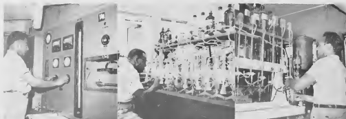
ERDCO FUEL coker simulates jet plane fuel feed system analysis in F. Ho Sam Sooi of Lab. No. 2.
